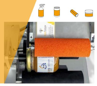
If front and back labels are on one label roll, the system can also place several labels on the circumference. The distance between the labels can be adjusted in the PLC.
