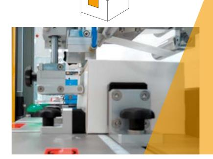
With the TNC-L model series, cardboard boxes and small cartons are provided with sealing or closure labels. The system can be infinitely adjusted to different formats.
