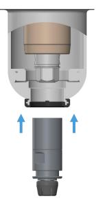
To remove the Bit holder from the screwdriver's shank, follow the bullets below:
