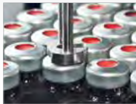
Press-fitting sealing plugs
