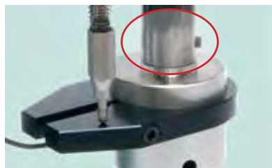
Ram with internal bore and grub screw
