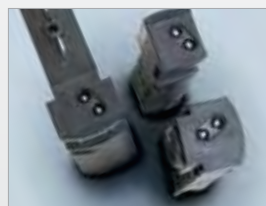
Inserting balls to seal holes
