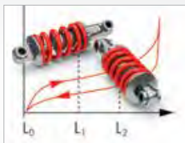
Spring testing with hysteresis monitoring
