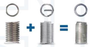
The **HONSEL COIL** "cone" can be installed in the same way as a coil with tab. No additional or special tools are required for process-reliable installation. When the **HONSEL COIL** "cone" is screwed onto the installation spindle, the conical portion of the wire thread insert creates a clamping effect between the installation tool and the coil. This ensures a stable installation process into the work piece.
