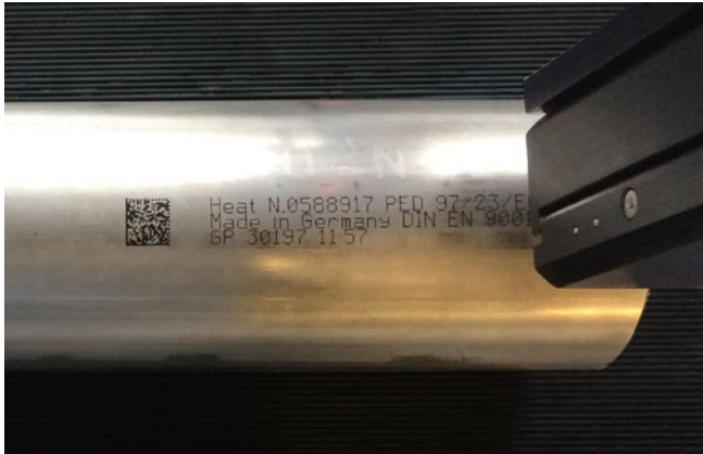
Coding and marking of steel pipes
