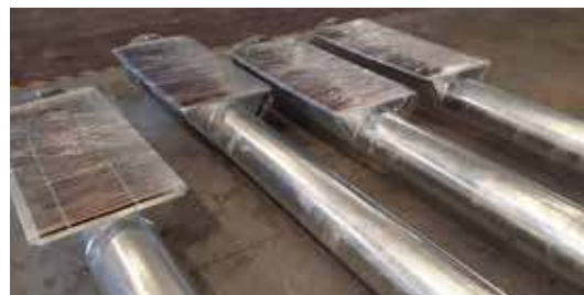
Tubular conveyor with hopper
