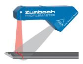
The measuring principle is based on 2D laser triangulation respectively light-sectioning technology. Four or more lasers illuminate the product surface and the associated matrix cameras capture the light contour from an oblique angle. A powerful and fast computer and the PROFILEMASTER software combine the captured segments into an orthogonal profile cross-section.
