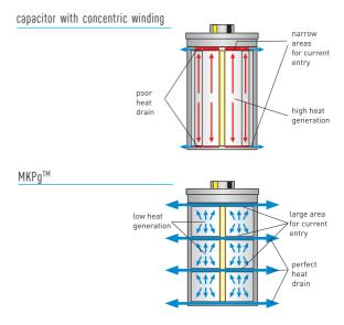
All the above features help to dramatically reduce the risk of field problems and premature capacitor failures. The MKPg is - by its principal design, superior know-how and matching dimensions, as well as by its careful workmanship (100% Made in Germany) - the ideal capacitor not only for your new projects, but also as retrofit for existing installations.
