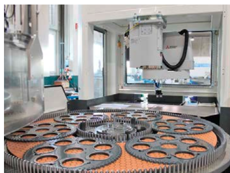
Robot Cell for automatic loading and unloading of the machine – also combinable with Twin Loader
