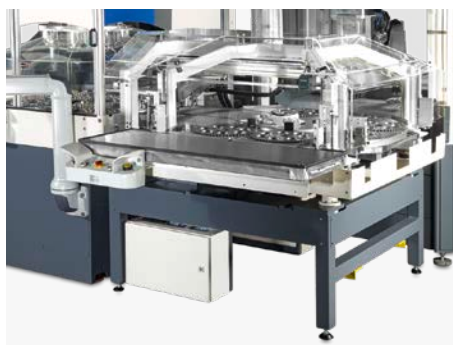
Twin Loader – automatic work piece carrier exchange for shortest loading times
