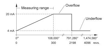
Note: If the measuring range cannot be found directly due to sensor shaft rotation (as the sensor system is in the overflow or underflow range), the rotary encoder can be pre-set with the aid of the MFPs. As a result, the rotary encoder jumps to the centre of the measuring range.
