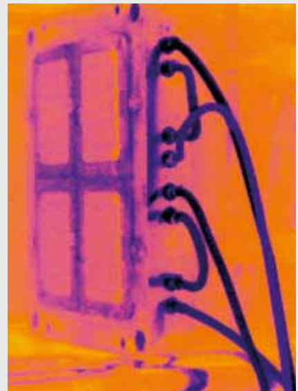
Homogenous temperature distribution in the injection mould after the temperature conditioning circuits have been cleaned.
