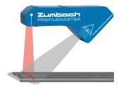
The measuring principle is based on 2D laser triangulation respectively lightsectioning technology. Four or more lasers illuminate the product surface and the associated matrix cameras capture the light contour from an oblique angle. A powerful and fast computer and the PROFILEMASTER software combine the captured segments into an orthogonal profile cross-section.
