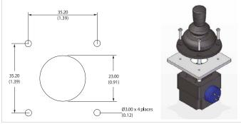
The joystick is mounted from below. The rubber bellows is guided through the hole in the mounting plate and pressed against the front. The screw connection is made through the cover.
