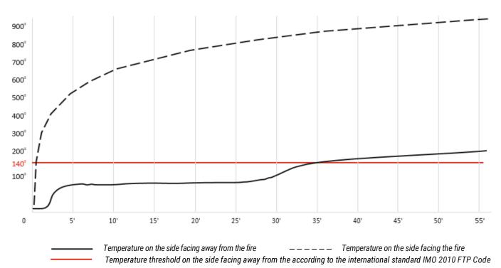
The essence of CBG-SeaPan is that the sandwich panel has a surface layer of multi-layer non-combustible basalt glass ceramic laminate on both sides. The core material consists of specially prepared mineral wool. All layers of this sandwich structure are bonded together by means of an inorganic nonflammable adhesive "LR Cerammatrix 01-50" with endothermic effect.
