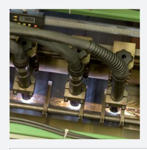
Plasma welded edges assure a continuous and frictionless passage of the filter sieve belts.
