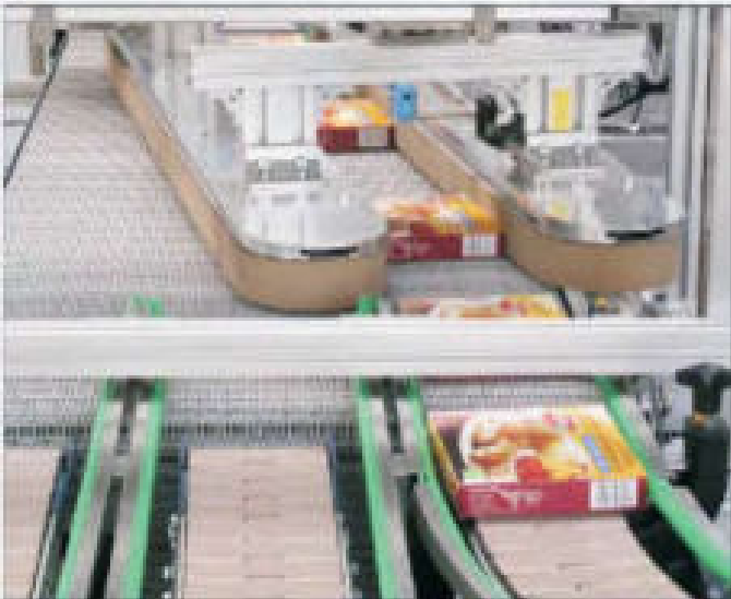
Motorized switch for uniform distribution on multiple tracks
