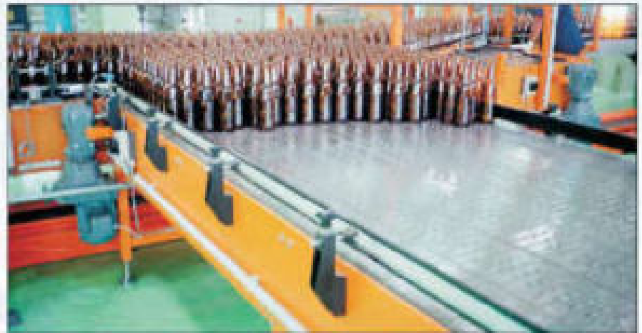
Stationery table in reverse operation
