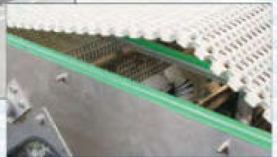
Integrated chain cleaning station
