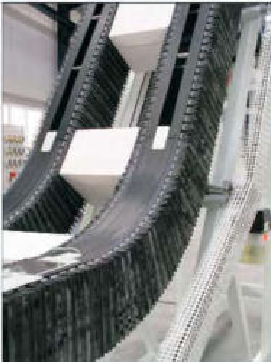
Wide gripper chain for heavy packages
