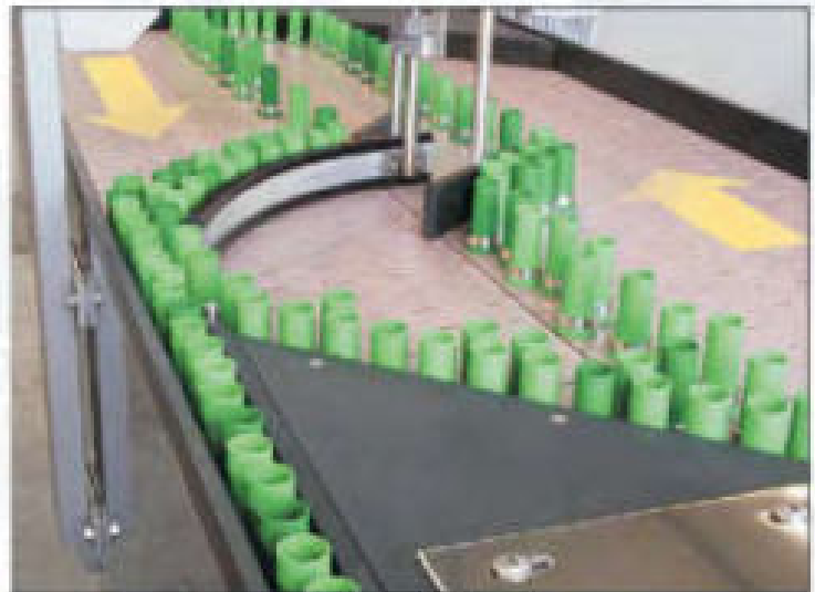
Stationery table in rotary operation
