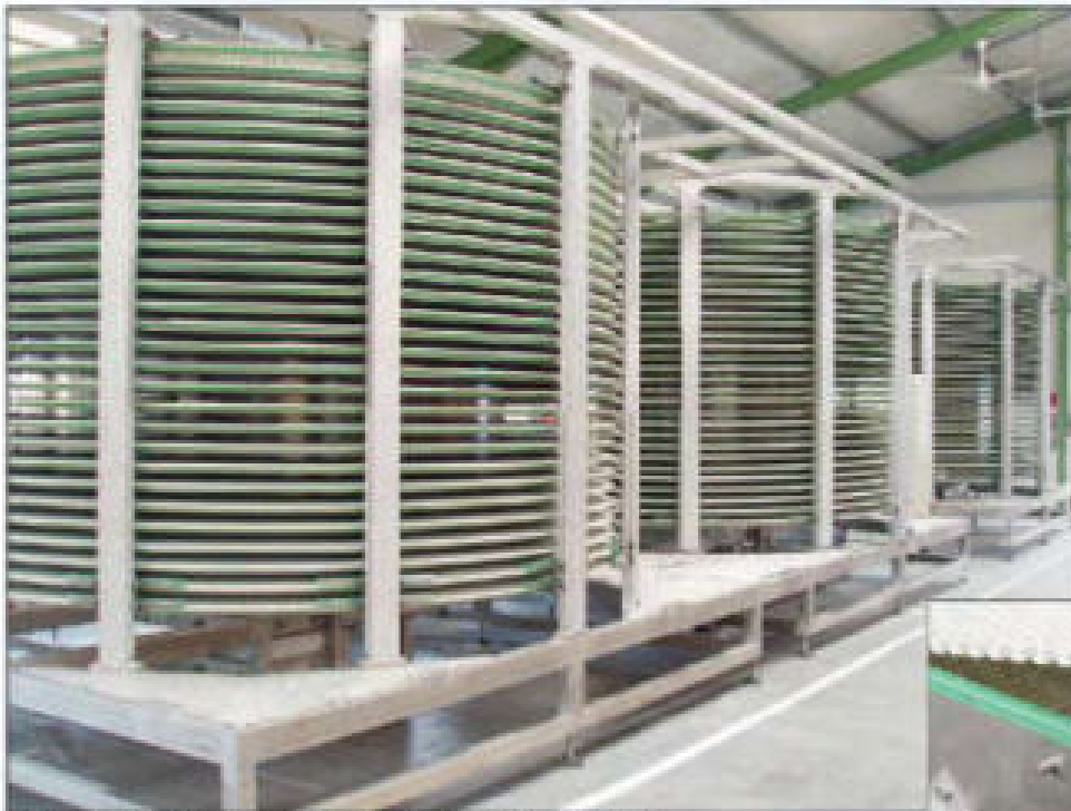
Three tower system with over 1200 m chain length
