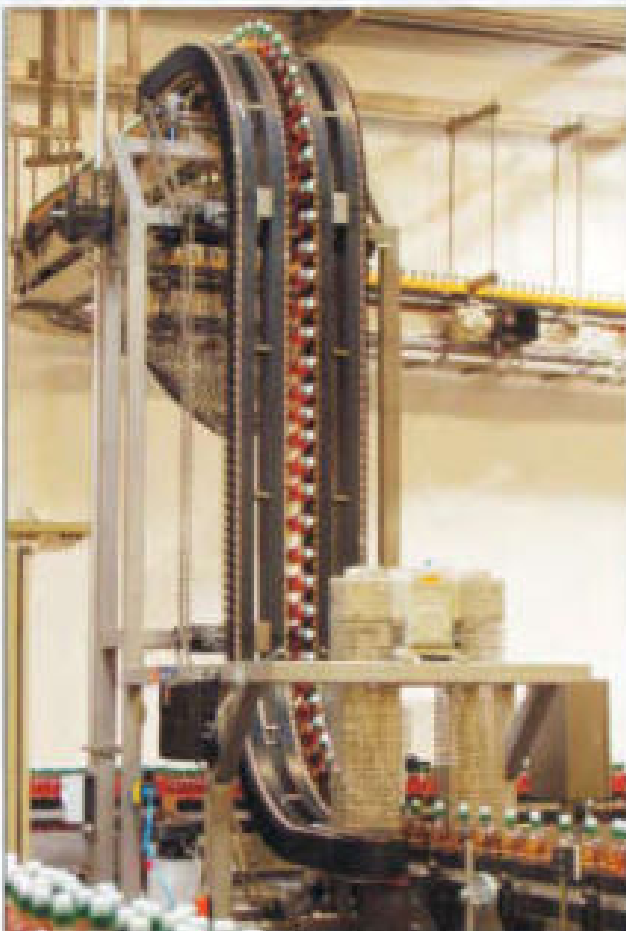
Downward transport of fruit juice-PET-Bottles
