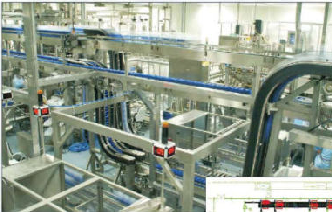
Compact conveying system in clean room conditions
