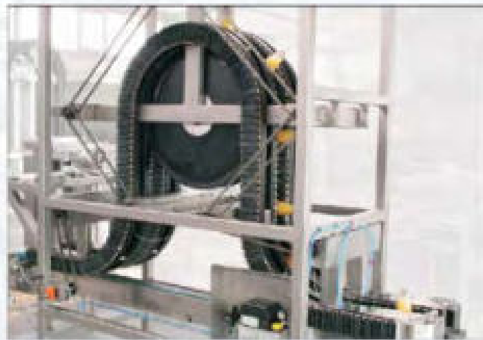
Neck sterilizer with revolving disk to reduce wear of chain and wear strips
