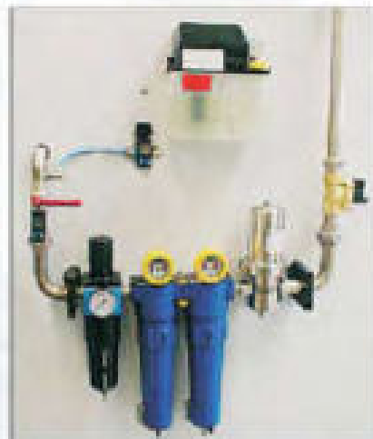
Sterile air filter unit and centralized lubrication system
