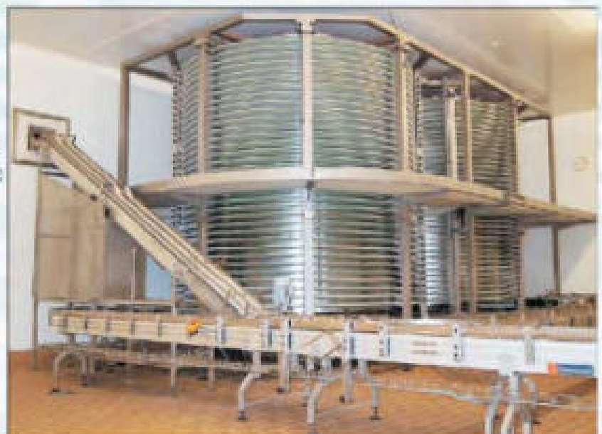
Spiral flow system with circulating gallery
