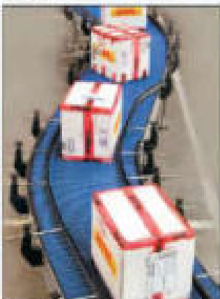
Modular belt conveyor with rotary device
