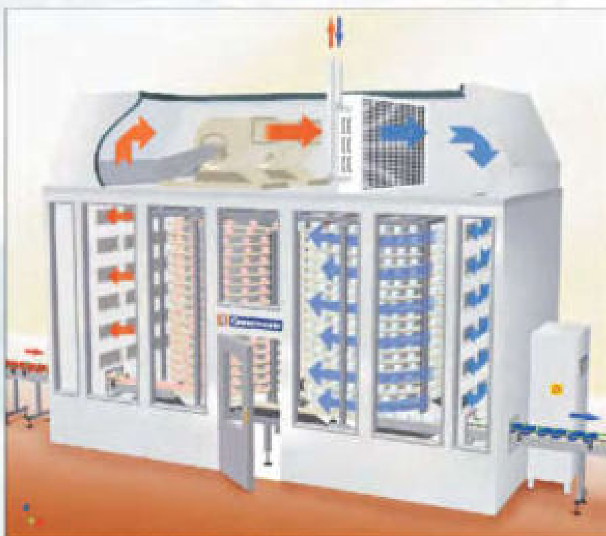
System scheme of spiral flow cooler
