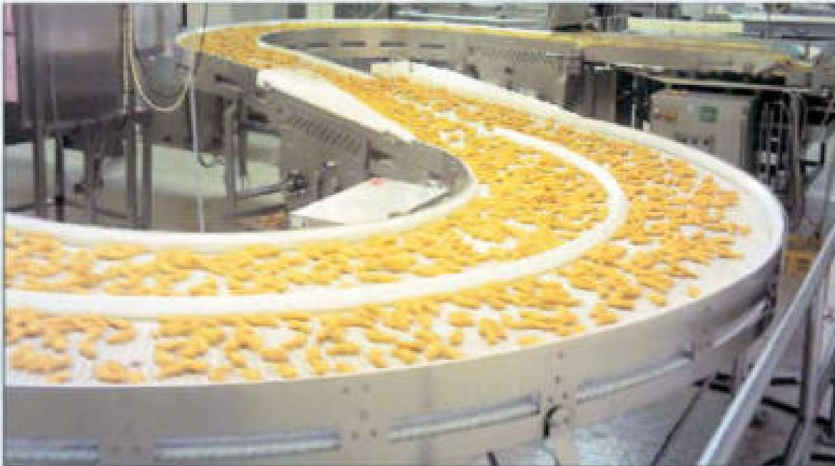
Modular belt conveyor in hygienic design
