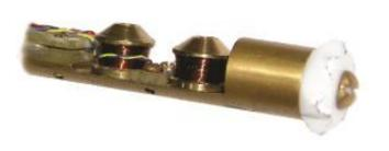
coils. The sample is placed into one of the coils (a measuring coil), the other coil (a field coil) is used to measure the magnetic field strength. The signal taken from the measuring coil is proportional to the magnetization and is induced with a change of the external field. It is recorded continuously simultaneously with the signal from the field coil proportional to the external magnetic field strength magnitude.
