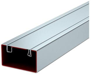
Four-sided, metal fire protection duct to install and route cables. With intumescent inner lining. In the event of fire, it prevents the spread of fire in the duct and protects emergency and escape routes against the impacts of a cable fire.
