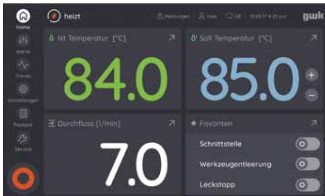
Display and control unit logotherm with user-friendly 7-inch touchscreen
