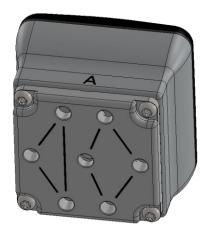
To mount the Adaptor Plate simply remove the 4 fittings or blinding screws from the gripper, place the Adaptor Plate by choosing the right angle according to the desired configuration, and tighten the 4 screws with 4 Nm tighten torque.
