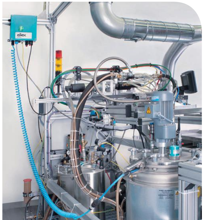
Active grounding for containers or drums
