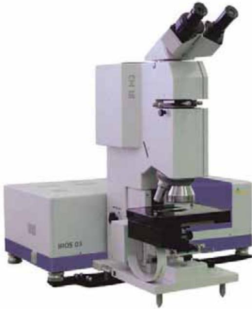
IR M3 high-end wide-range IR microscope
