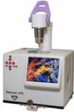
Multi-purpose ATR/SDR module
