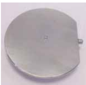
Sample holder with diamond prism
