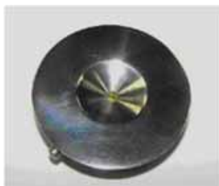
Sample holder with ZnSe prism
