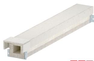
The fibre glass light-duty concrete ducts, which can be flamed on four sides, can be mounted on OBO mounting systems, thus offering the greatest possible flexibility in cable routing in emergency and escape routes (installation duct to DIN 4102 Part 11) or in the maintenance of electrical function (to DIN 4102 Part 12). This allows elegant avoidance of objects from other areas such as heating, ventilation and sanitary applications.
