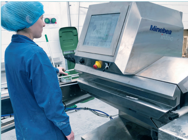
The X-ray inspection system Dylight reliably detects foreign bodies in product processes
