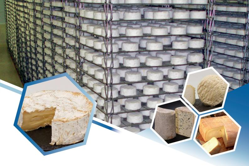
The space between the wires allows a good air circulation Excellent oxygenation of the cheeses and regularity of the ageing process The racks ensure support and ventilation of the products
