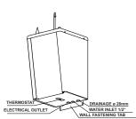
Installation by means of three basic connection points.
