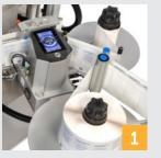
Featuring a wrap-around belt and a counterpressure plate, the machine is suitable for a very wide range of cylindrical products.
