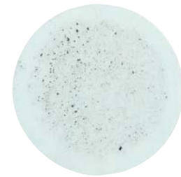
Cleaned with compressed air
