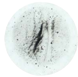
Residual particles from a hydraulic hose, not cleaned
