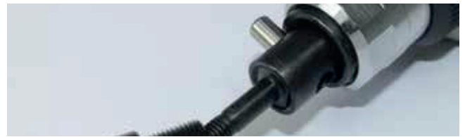
Quick-change system for the threaded mandrel.
