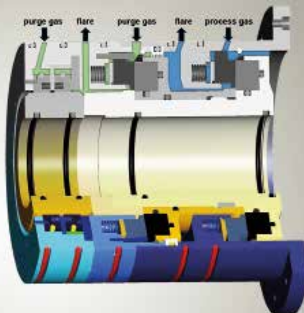
Fig. 1: Tandem seal with intermediate labyrinth
