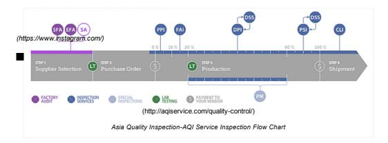
The During production Inspection (DPI) provides a quality check, normally for the first time of the finished products. It ensures that all processes and products are being produced to the agreed standards and timeframes.
