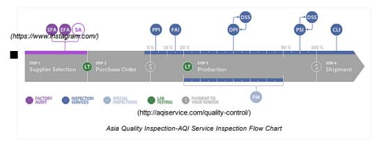
The First Article Inspection (FAI) attests that all engineering, design and specification requirements are rightly understood, accounted for, verified, and recorded.
