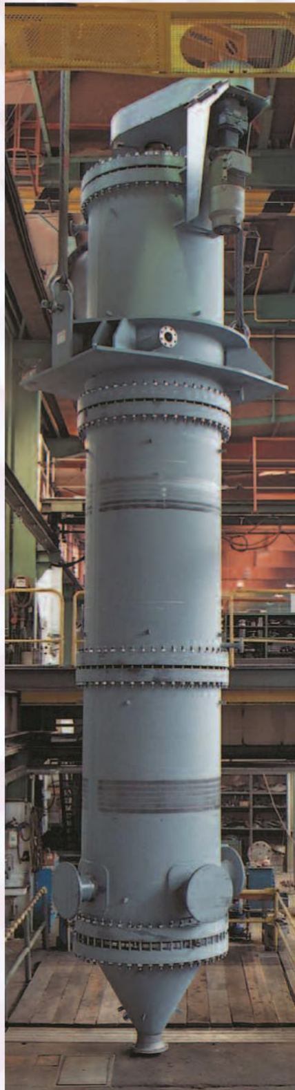
Thin film evaporator in our test facility
