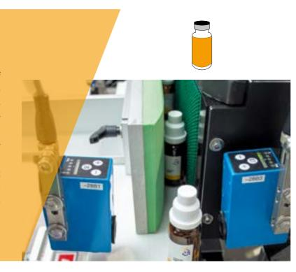
Both the vision system and the print engine are fully integrated in the touch panel HMI. Shift registers in the label applicator as well as in the complete system enable product and label tracking through the complete system.
