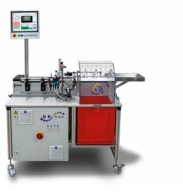
This powerful HSF friction feeder is the optimal solution when empty folding boxes have to be marked with variable data offline from the production line. The modular design of the system enables an easy integration of the desired marking technology.
