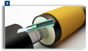
The surface is cleaned off from the dirt and trimming that occur after heating.
