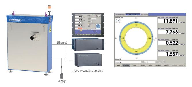
The USYS IPC 1e/2e processors allow complete process control and optimisation. All measured values can be monitored and logged by the software. The stored product recipes enable easy operation of the system. Additional sensors such as: ODAC laser diameter gauges or KW lump detectors can be connected if required. The USYS processors also has inputs and outputs for alarming the line control and can also communicate with a higher-level system via the HOST interface.
