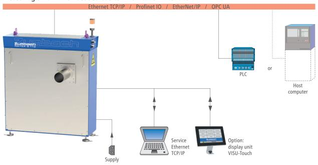
The design with embedded communication interface allows the higher-level system to configure and capture measurement results. The measuring algorithm itself is controlled by the RAYEX S and only requires the number of layers and the nominal wall thickness to be specified. All measurement results can be read and processed by the higher-level system.
