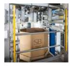
The semi-automatic big bag filling station makes it possible to fill big bags (FIBC - flexible intermediate bulk container) with one, two or four loops and octabins with a filling station of 500 kg to 1500 kg.
