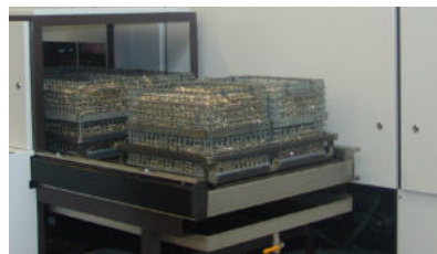
Goods carriers outlet, two-lane, double-layer
