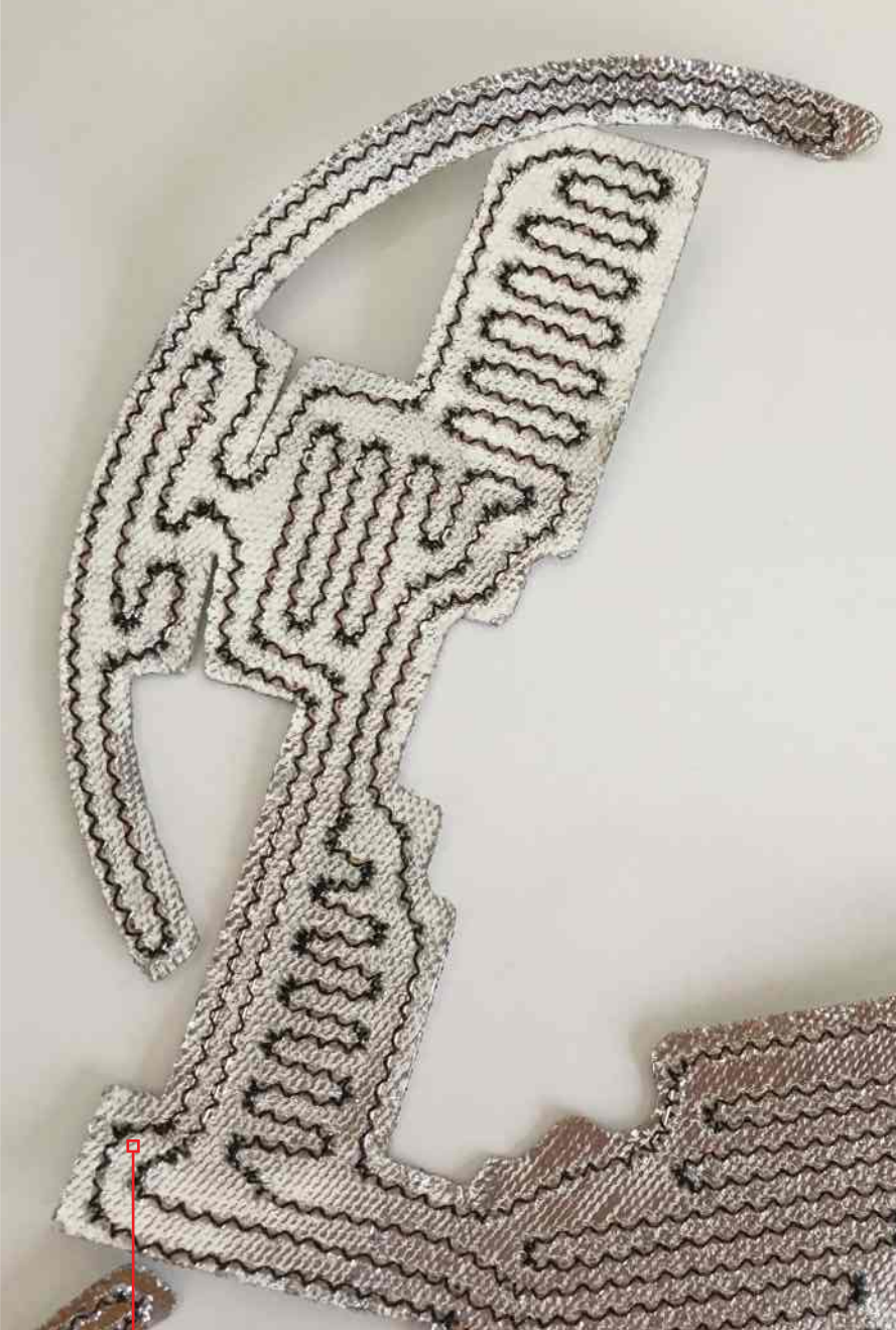
12V-heating element on a fabric made of aluminium with a ultraflexible steelbraid
