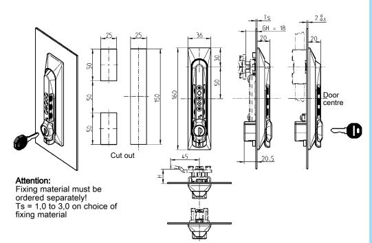
Swinghandle polyamide GF black, shaft zinc die zinc plated, with seal, round cylinder with stainless steel cap and shutter. Each round cylinder has one silver steel key with polyamide grip GF black.
