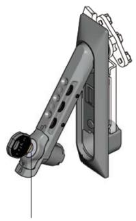
Option 1: Release using round cylinder, operation as with usual swinghandles of program 1150. The combination lock remains untouched.
