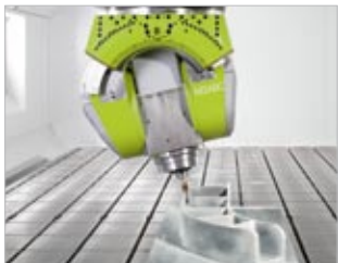
The unique third axis is clearly visible. This B-axis can be moved simultaneously by \pm 15^\circ .
